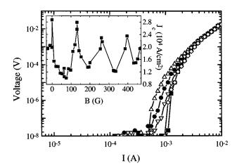
FIG. 4. I-V curves as a function of field at T=7.7 K for the  $100\pm10$  nm thick Nb film on top of the square array of Ni dots. The curves are shown for the following fields:  $0 \text{ G }(\blacksquare)$ , 10 G (Φ),  $64 \text{ G }(\triangle)$ ,  $110 \text{ G }(\nabla)$ ,  $132 \text{ G }(\diamondsuit)$ . Inset shows the critical current extracted from the I-V curves with a  $5\times10^{-3}$  V/m criteria.
