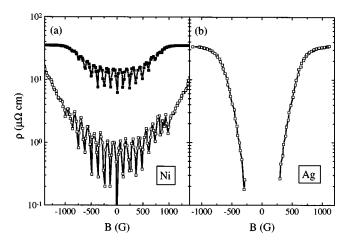
FIG. 2. Field dependence of the resistivity of a  $100\pm5$  nm thick Nb bridge on top of a square array of Ni or Ag dots with a lattice spacing of  $d=400\pm10$  nm. The applied current density is  $J=2.5\times10^2$  A/cm². (a) Two curves with temperatures of T=8.1 K ( $\blacksquare$ ) and T=7.9 K ( $\square$ ) are presented for the Ni. (b) For comparison, the curve presented for Ag was measured at T=7.9 K.
